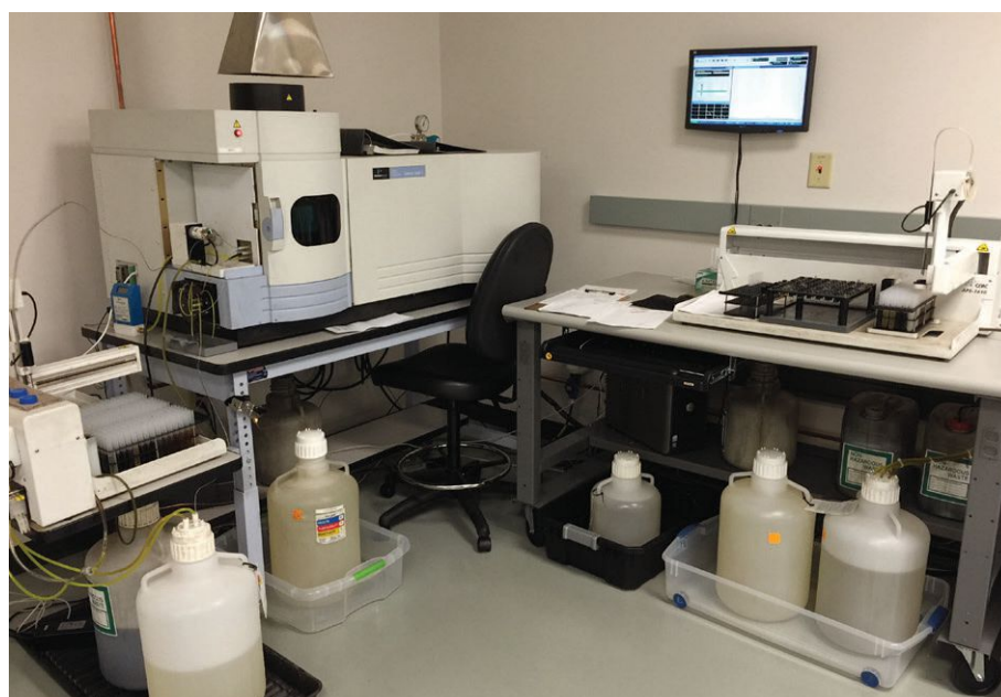
Figure 7 | An inductively coupled plasma unit identifies metallic elements in oil. (Photo courtesy of David Scott, Analysts, Inc.)
