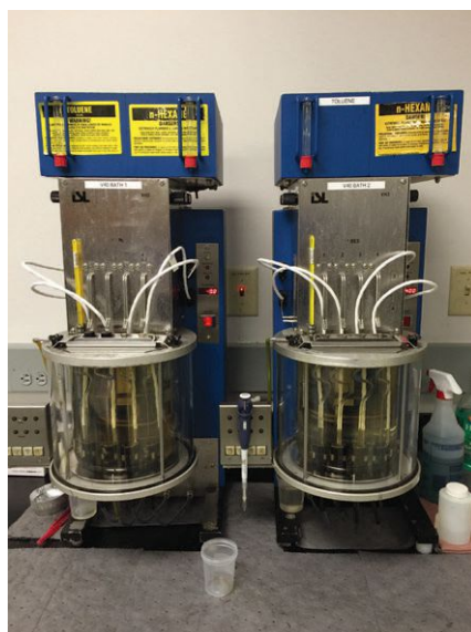
Figure 5 | Capillary tube viscometer measures viscosity at 40 C, a typical test for industrial oils. (Photo courtesy of David Scott, Analysts, Inc.)
