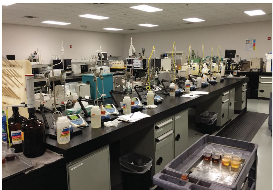
Figure 9 | Lab setup for measuring acid and base numbers. (Photo courtesy of David Scott, Analysts, Inc.)
